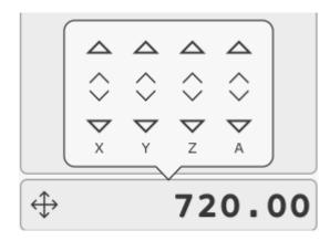
Mouse click+hold on large arrow jog buttons to jog machine in desired direction. Machine will move until the mouse button is released. Corner buttons allow diagonal or combined axis jogging.
