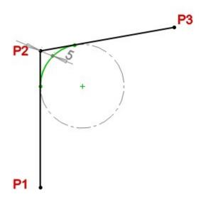
You can see that greater tolerance and/or smaller angle generates larger blend arcs. Moving on those arcs generates forces because of radial accelerations. Maximum radial acceleration is limited with settings "Motion/Max Acceleration" and "Motion/Max Deceleration".
