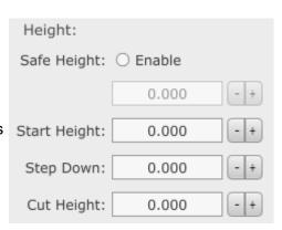
With this option enabled, generated toolpath will include traverse moves performed at safe height.
