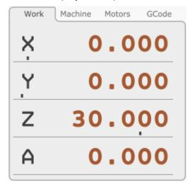
User can set new *Work/Coordinate System* position value by double clicking on the axis position value of Work tab. *To Value...* insert field will appear:
