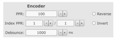
Sometimes we have multiple index sensors, typically on lathes, for example three index sensors will give you signal every 120deg of revolution. So the ratio in such case would be: **3/1**
