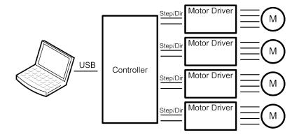
The PlanetCNC series of CNC motion controllers are link between a personal computer and motor drivers supporting step/direction control. They are compatible with most drivers. The controllers use the USB or Ethernet port, available on all modern computers and laptops. They can serve as direct replacement or upgrade for many parallel port break-out boards.
