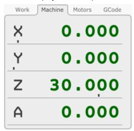
User can set new *Machine* position value by double clicking on the axis position value of *Machine* tab. *To Value...* insert field will appear:
